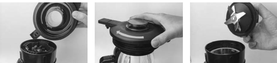
To assemble, the sealing ring is first attached to the blade unit. When doing so, make sure the sealing ring is properly seated on the blade unit. Place the locking base on the mixing container and turn it counter-clockwise as far as it will go.
