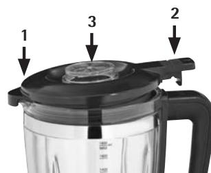
To this end, place the spout of the lid sideways against the pouring spout on the mixing container and gently press the lid onto the mixing container (1). Then press the locking mechanism on the lid downwards until it clicks into place in the handle (2).
